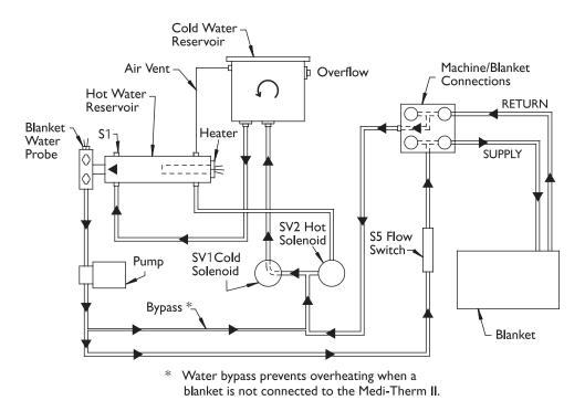
Figure 11—Cooling flow diagram
