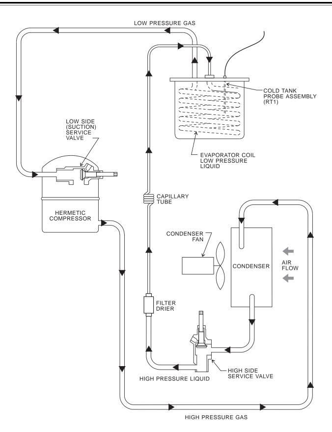
Figure 12—Refrigeration flow diagram
