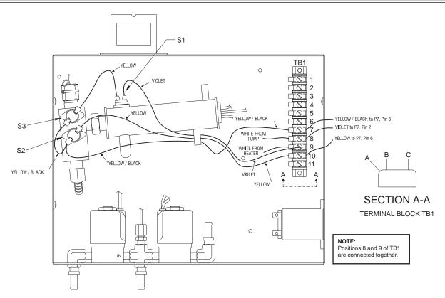
Figure 17—Original Thermostat Wiring Diagram for MTA5900/MTA5901
