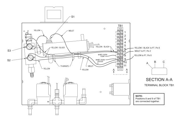
Figure 17A—New Thermostat Wiring Diagram for MTA5942 & MTA5900/MTA5901
