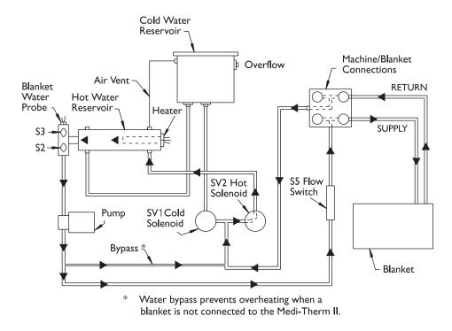
Figure 10—Heating flow diagram
