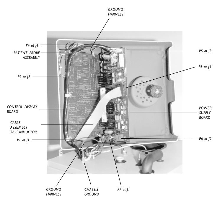
Figure 8—Circuit Boards and Connectors (Head)
