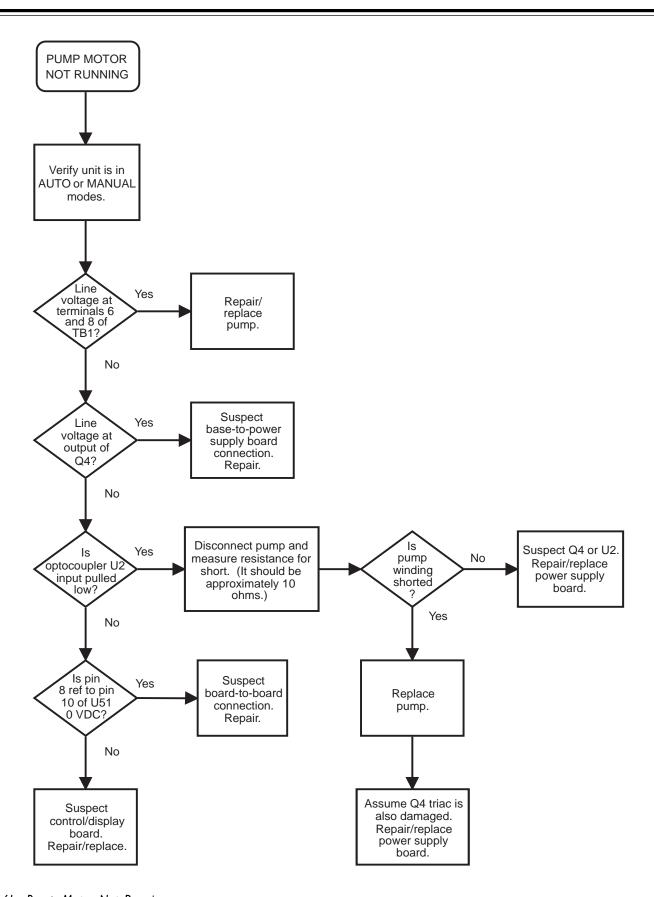
Figure 6J—Pump Motor Not Running
