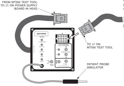
Figure 4—MT590 Test Tool
