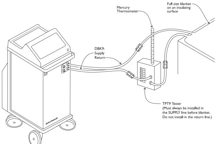
Figure 13—Test setup
