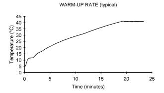
Figure 1—Typical warm-up rate (with full size blanket)
