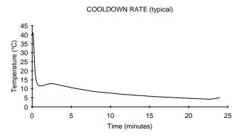
Figure 2—Typical cooldown rate (with full size blanket)
