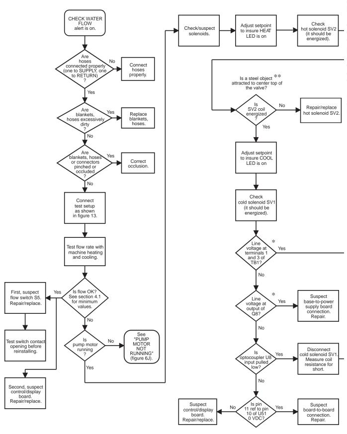
Figure 61—Check Water Flow Alert is On, Page 1 of 2
